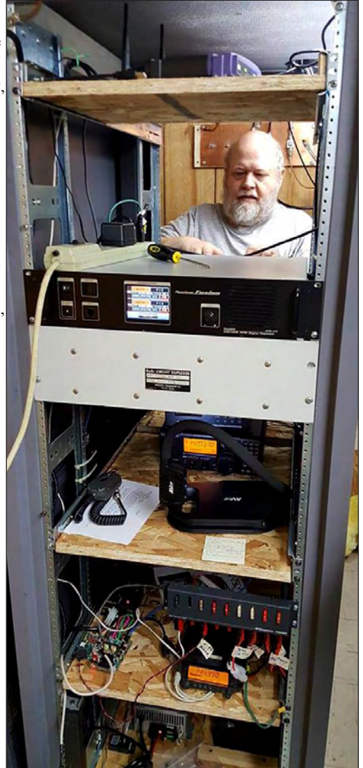
Erik Brom, WBØNIU, makes connections for the club's second Yaesu Fusion repeater.
